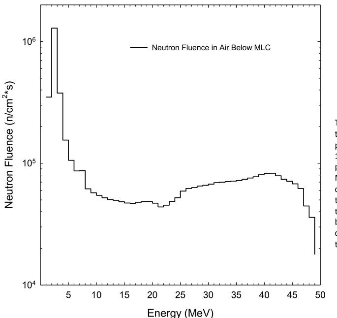
The fluence was tallied across a plane that was 100x100 cm^2 placed below the MLC in air (131.35 cm from the top of the beryllium target). Fluence based on a proton current of 66 uA on target.
